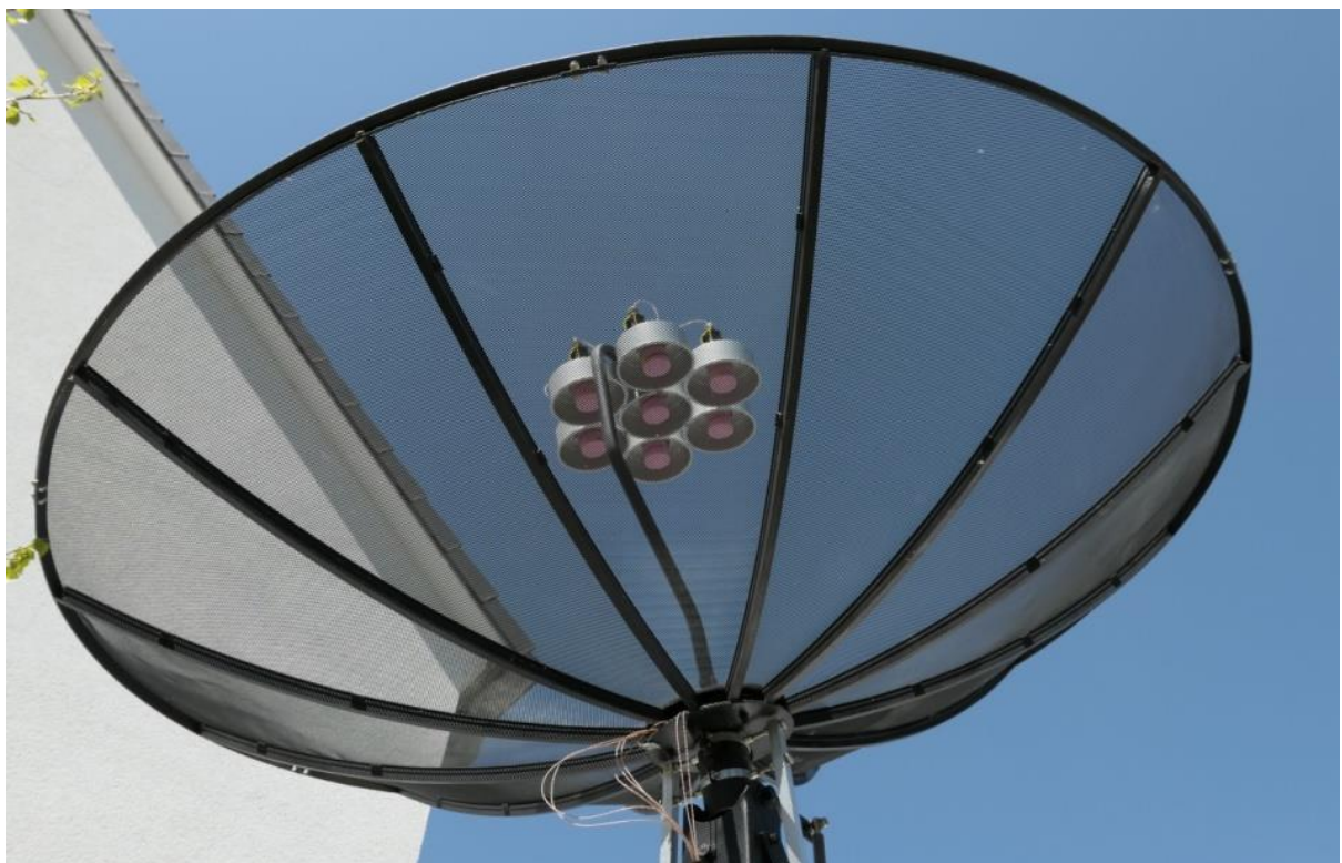
Robotic 2.6m radio antenna dish with seven HI-feeds (21cm) for successive meridian scans in order to compose seven slightly different sub-pixel-shifted lowRes images of the radio sky
